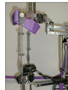
Enhanced steering mechanism allows 0 to 360 degrees of control and unilateral adjustment.
